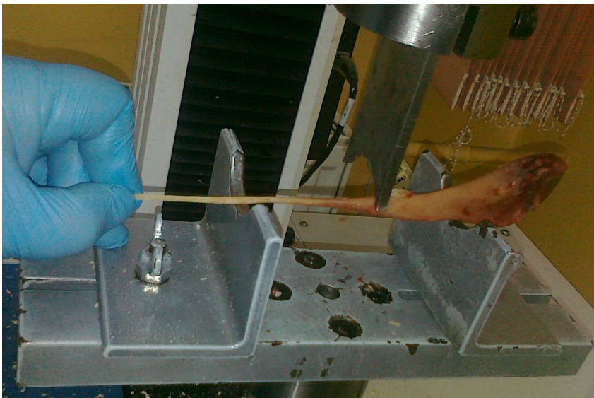
Fig. 4. The placement of fibula on bone supports during the three-point bending test in an Instron 3367 apparatus (Instron, Canton, MA, USA). The measuring head loaded fibula on the posterior surface with constant speed of 50 mm/min.
